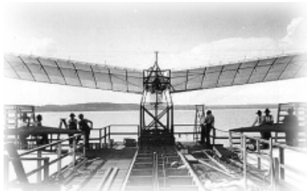
Langley's "Great Aerodrome" perched aboard a houseboat on the Potomac, just before a disastrous launch that tumbled the aircraft down into the river.
