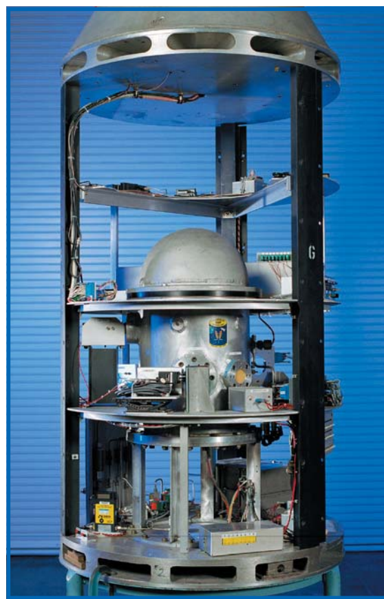
Drop vehicle with gas jet combustion experiment onboard.
