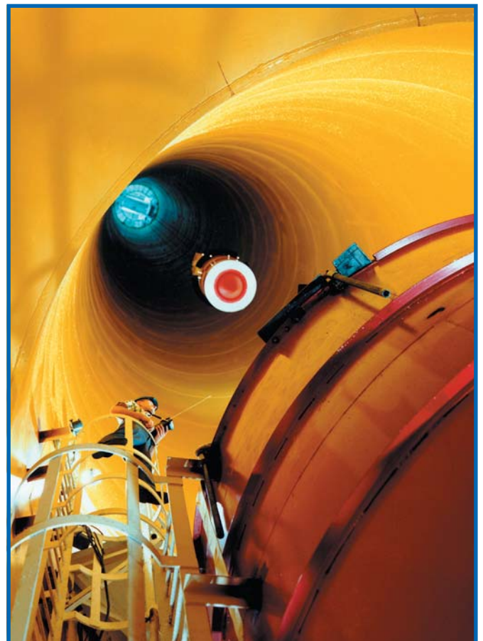
Retrieving the drop vehicle after a test in the Zero-G Facility.
